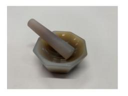
Ideal for grinding samples e.g. prior to melting point analysis.
