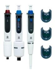
Brand Transferpette® S Starter-Kit Macro: 3 x Pipettes - 100-1000ul, 500-5000ul, 1000-10000ul, 3 Shelf Mounts
